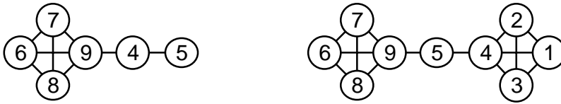
FIG. 2.4. On the left, the elimination graph G_{\{1,2,3\}} ; on the right, a perfect elimination ordering generated by the algorithm.
